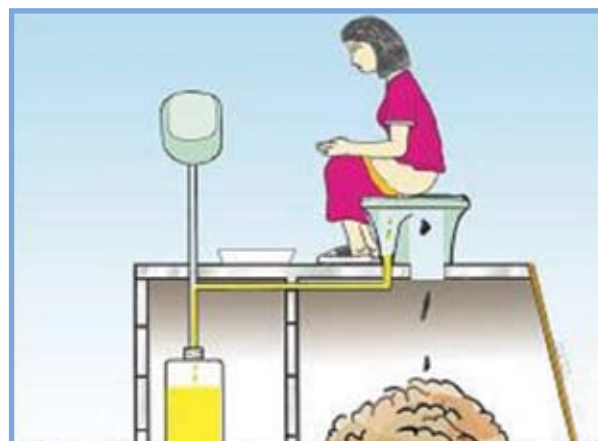
Ecosan toilets promote the separation, collection and reuse of feces and urine for agricultural production.
